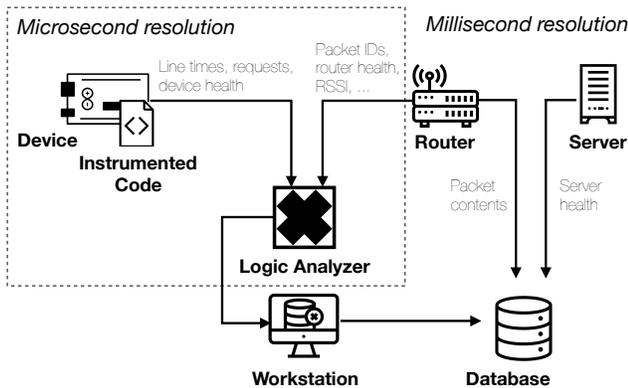
**Figure 9.** Dataflow through the WiFröst network components. Logs are collected from instrumented code, device, router, and server. The method of data collection varies by the time resolution required to preserve causation between events from neighboring components.
