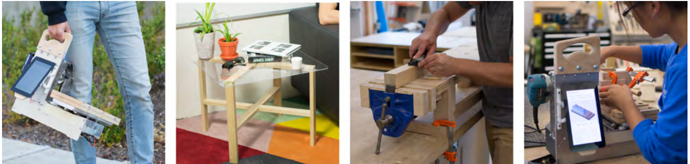
Figure 1. MatchSticks is a new digital fabrication system for woodworking (A). Wooden objects larger than the size of the machine can be easily made using a parametric joint library (B and C). We evaluate our system with users (D) who followed an on-screen tutorial to create a parametric box.
