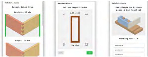
Figure 7. The web application's user interface for selecting the joint type and inputting the size of the stock.
