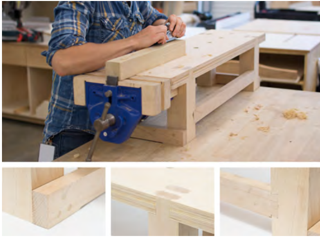
Figure 12. In traditional woodworking, a large flat piece of wood can be difficult to source or construct, requiring a variety of specialized tools. In this example, we use plywood for the tabletop and maple lumber for the components of the legs, demonstrating the complementary capabilities of traditional CNC routers and our tool.
