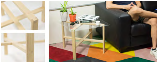
Figure 11. Three styles of joints (X, T, and L) are used in combination to create this table. All pieces used in this table are longer than any dimension of our CNC tool.
