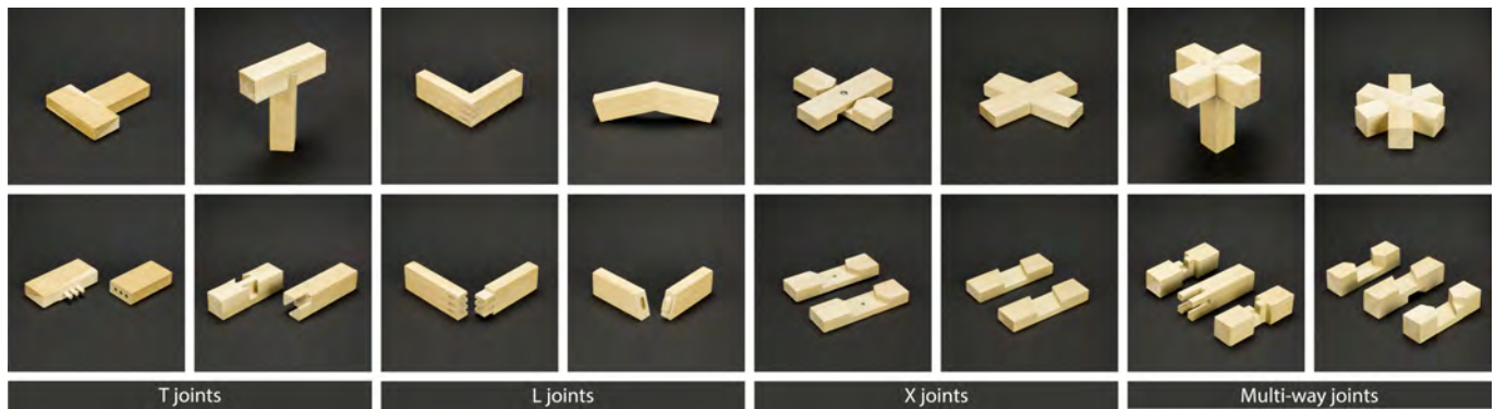
Figure 8. We categorize the joints our machine can create based on the orientation in which they come together. Top row shows assembled joints, bottom row shows disassembled joints. From left to right: dowel pin joint, framing joint, finger joint, angled mortise and tenon, pivoting lap joint, angled lap joint, three way interlocking tenon joint, and three way lapped joint. All example joints are created from poplar.
